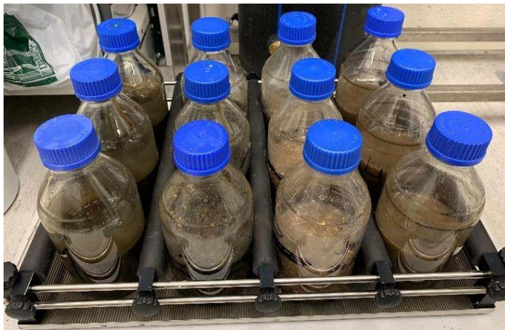
Figure 1 Laboratory-scale VFA production bioreactors (Articles I & II).
